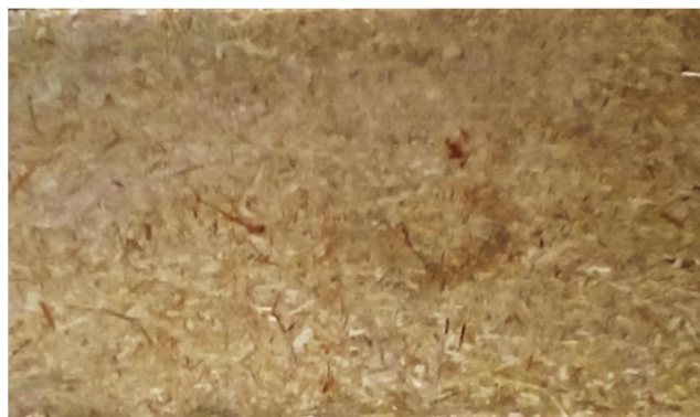
Figure 8. Particleboard of Andropogon gayanus stems.
